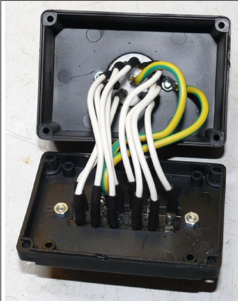
Wiring with stranded wires.
