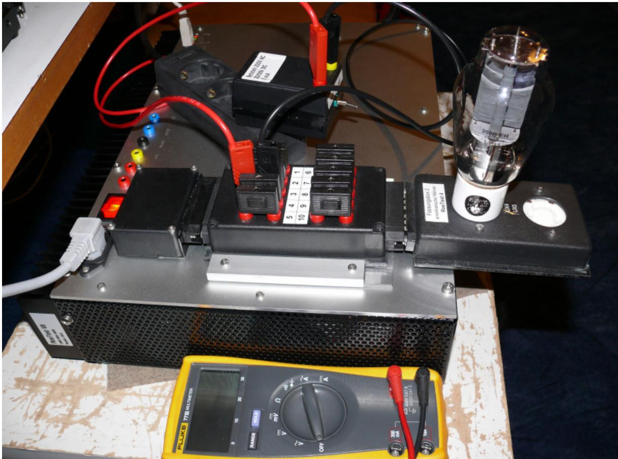
With the 300b the grid is located at pin 3. So we loop-in the external 60V there. The negative pole is connected to the tube and the positive pole is connected to the RoeTest. With a multimeter the sum voltage (internal grid voltage of the RoeTest + external power supply unit voltage) can be monitored.
