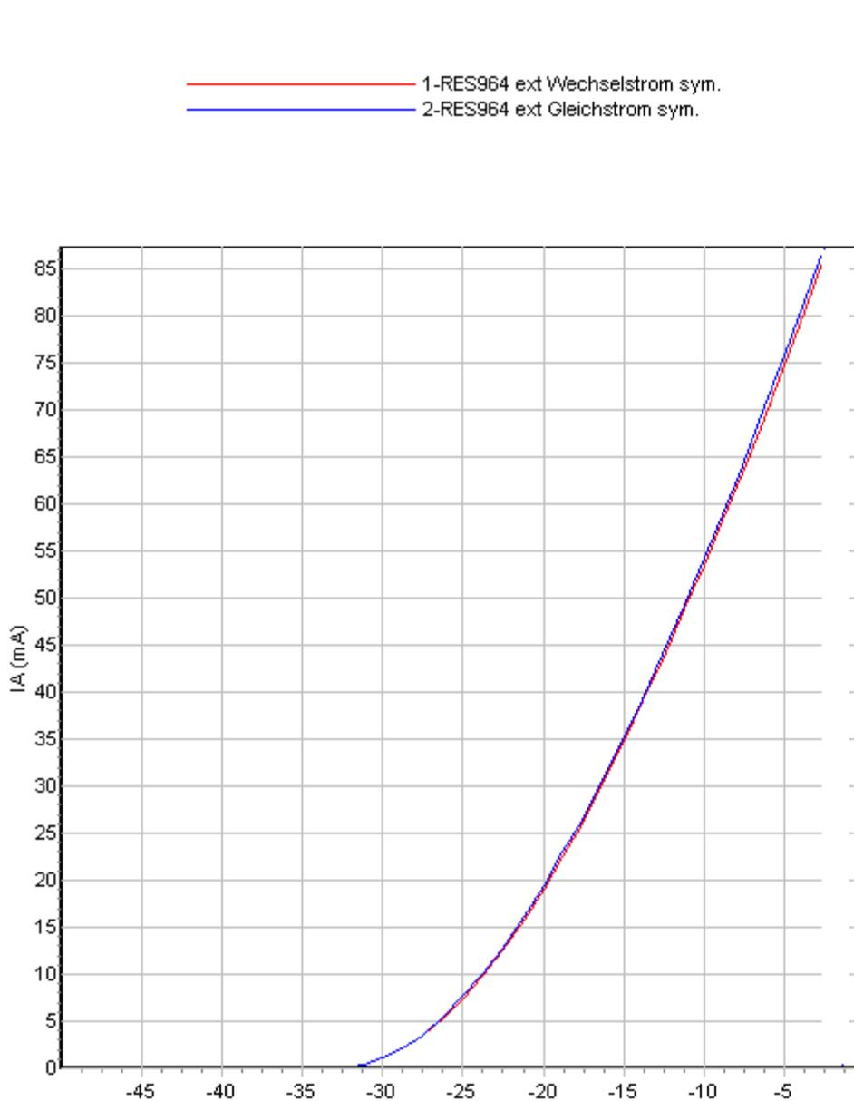
Result: The characteristic curves are identical. The claims from above are confirmed. From this results follows that in practice it does not matter if the tube is heated using AC or DC current as long as the circuitry is identical. If there are differences at all these are so small that they can be neglected.
