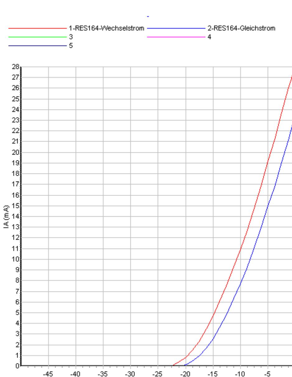
Result: When using DC heating (blue curve) the anode current is somewhat lower compared to AC heating (red curve). The characteristic curve is evenly shifted to the right.
