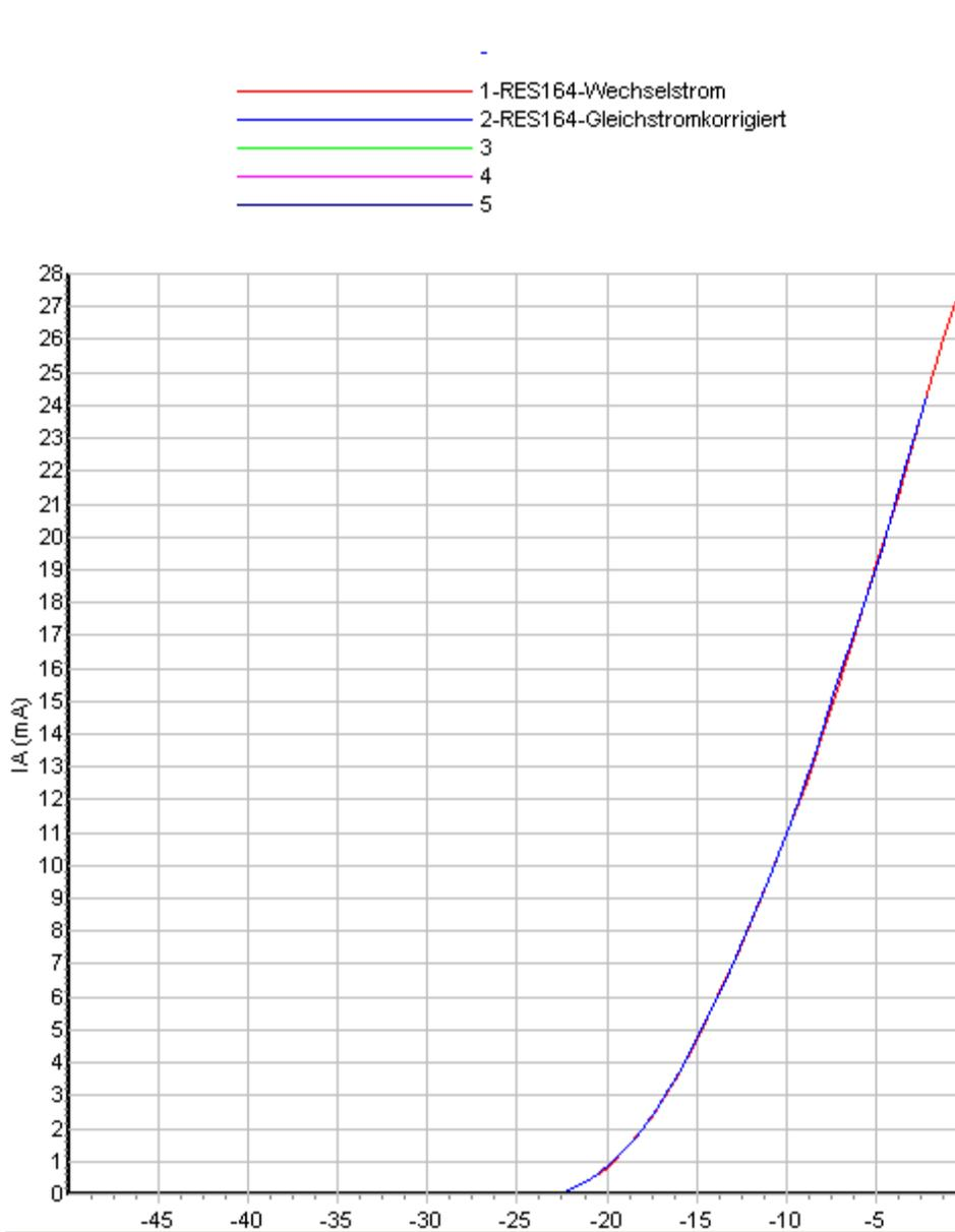
Result: The measured characteristic curves are identical for AC and DC heating and merely shifted to the right (lower values) when using DC heating.
