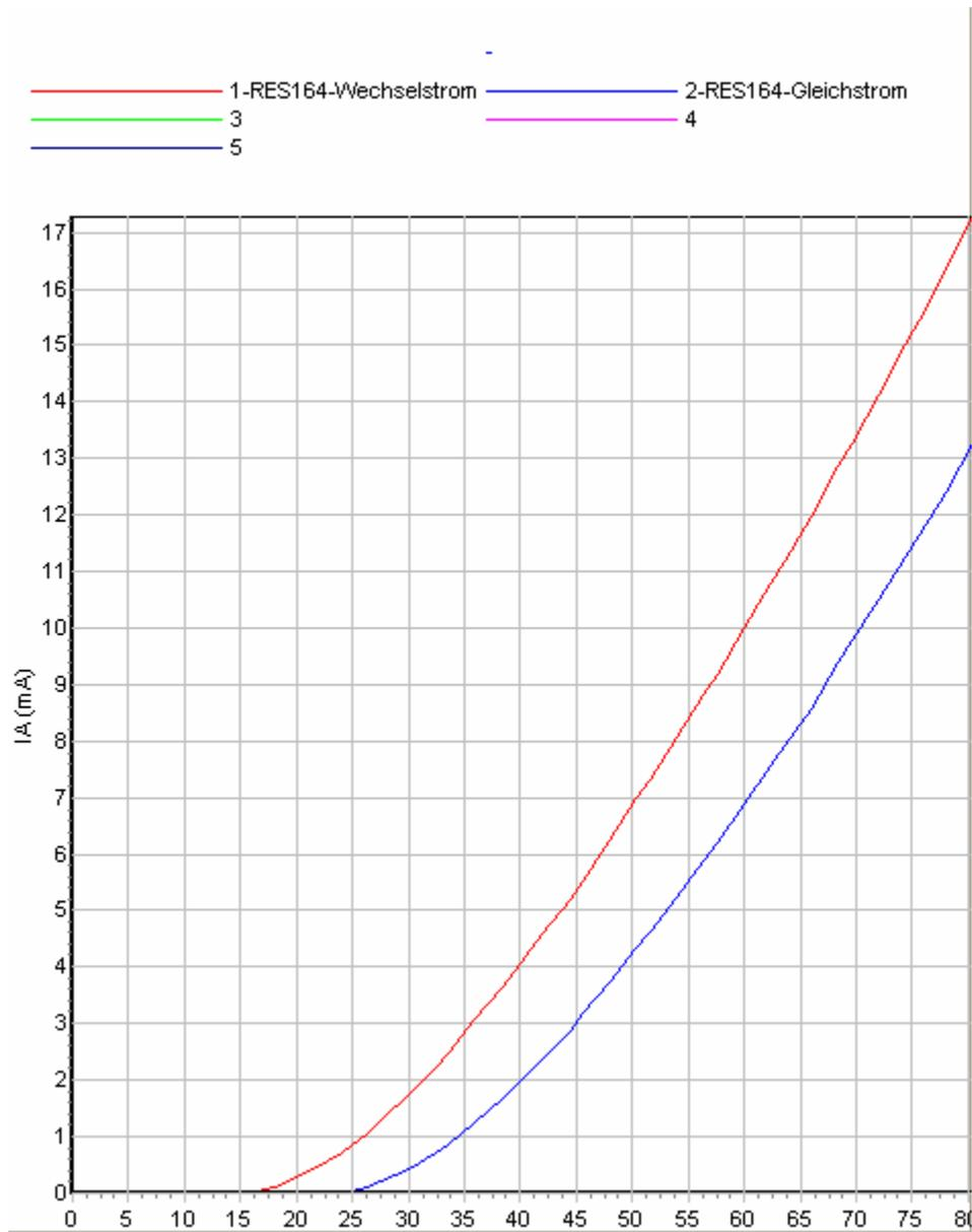
Result: As already seen with the G1 characteristic curve the anode current of the G2 characteristic curve is lower at DC heating compared to AC heating. The characteristic curve is also shifted to the right.
