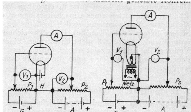
With AC heating the same potential is located along the filament (seen from a DC view point). The voltage swings around 0 volt (from maximum to zero and then to the minimum).
