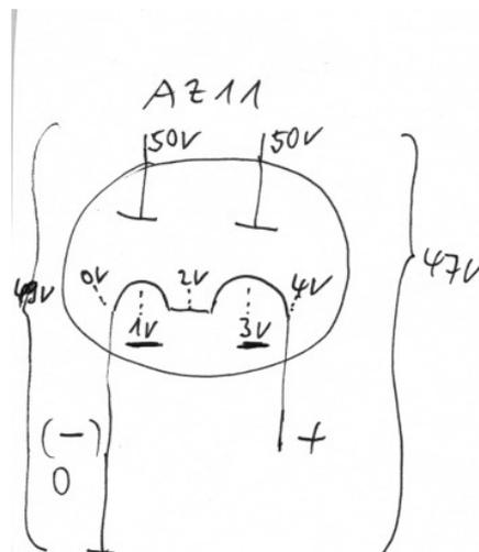
At the left system the filament in average has a potential that is 1V higher measured against ground. The right system in the example above there is a potential that is 3V higher.
