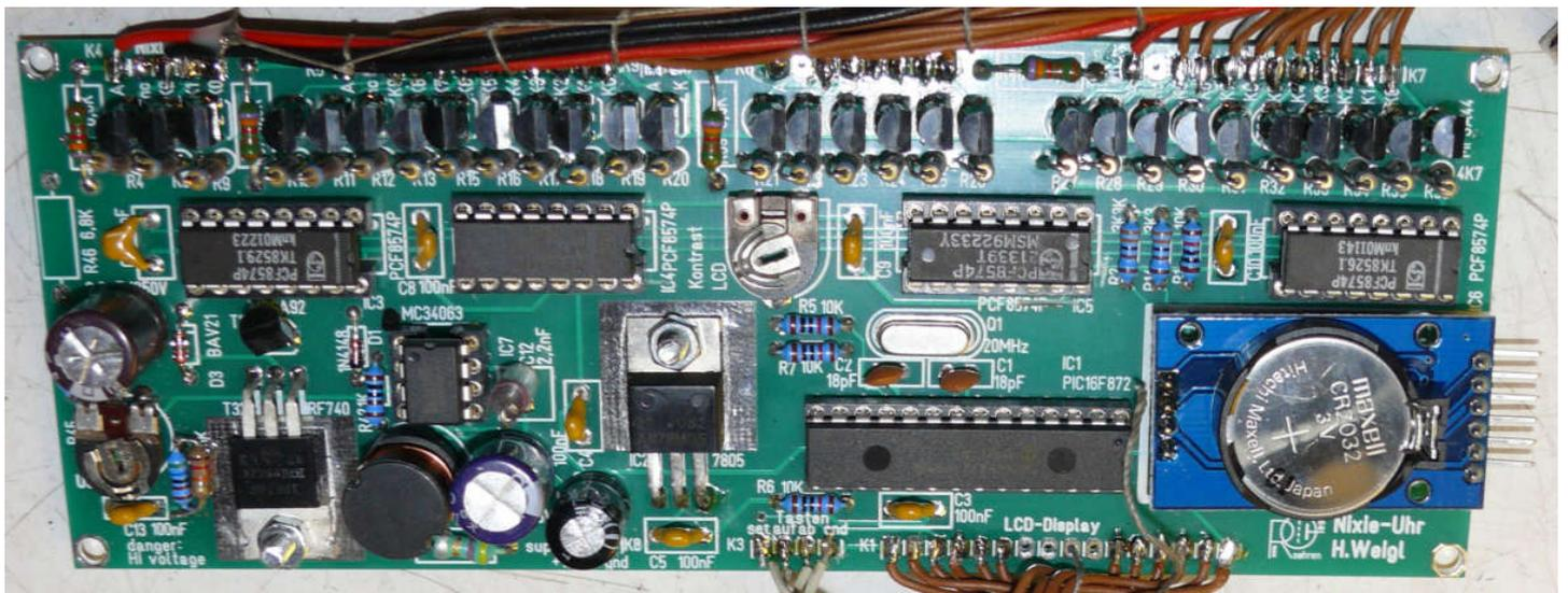
On top are the connections for the Nixie tubes. Only the required driving transistors were implemented (the ten's of the hour display only needs the digits 0-2, the ten's of the minute display only the figures 0-5).
