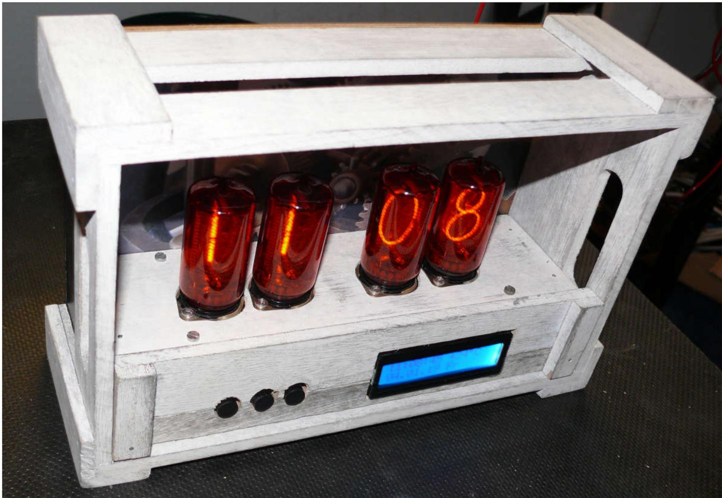
At last I managed to build a long planned project, a Nixie tube clock.
