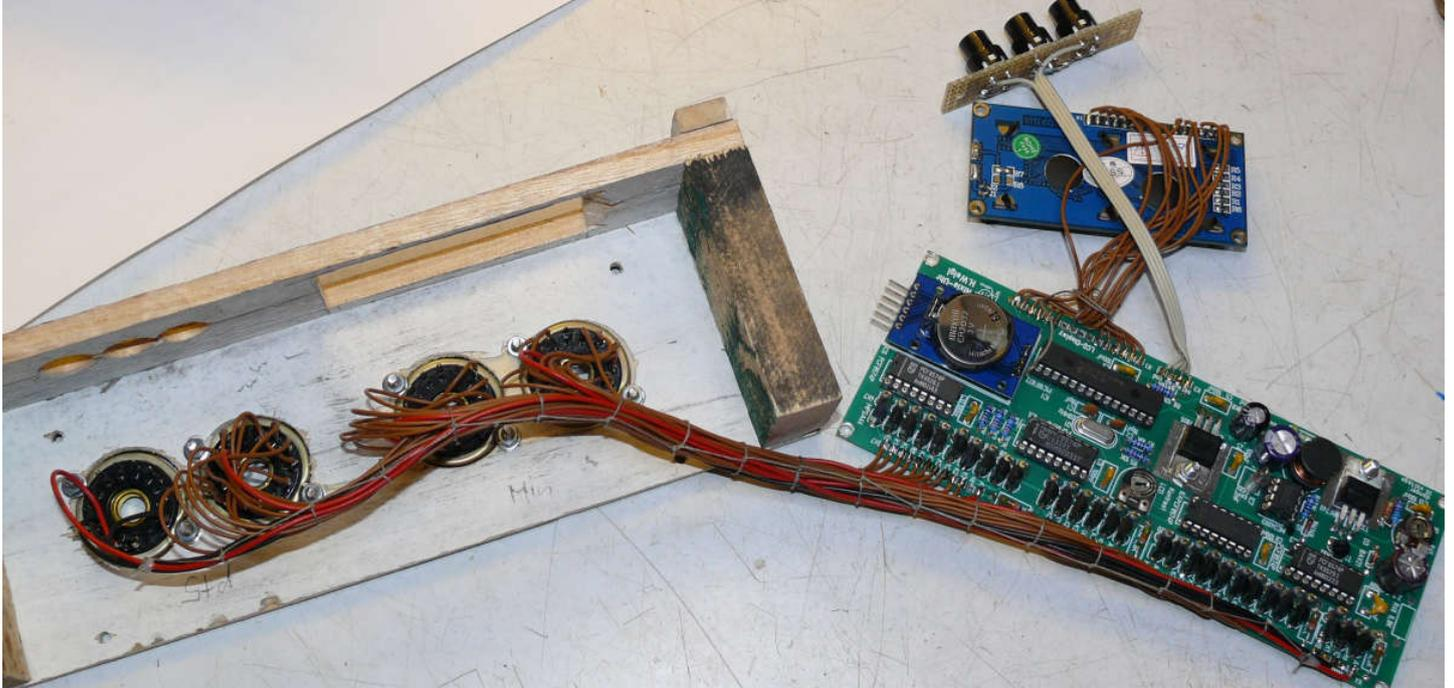
Unfortunately ('as usual') an error occurred on the circuit board's prototype. The VDD and VSS pins of the PCF8574 are transposed. Therefore some tracks had to be cut and wire bridges had to be inserted:
