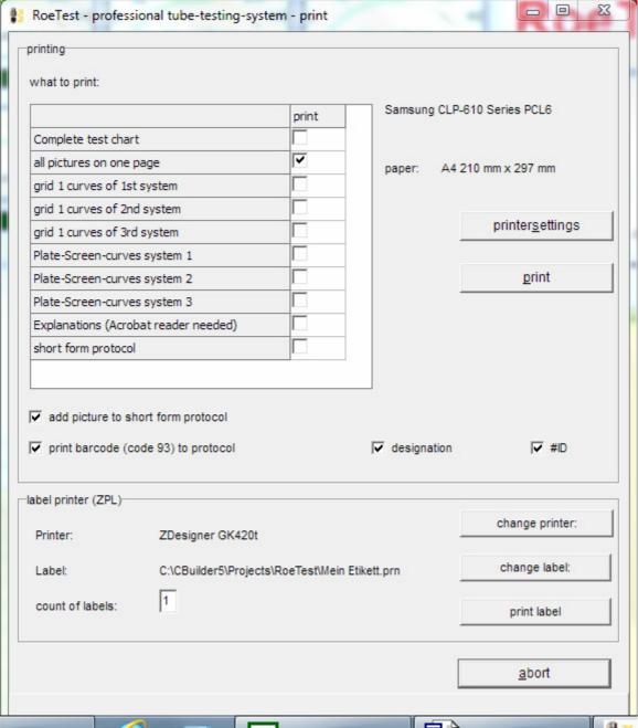
The RoeTest offers printing of a complete protocol as well as only printing the graphics, an annotation or (new) a short protocol.
