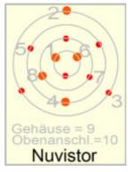
New numbering: The pins most often used/lead through to the outside are drawn in orange. The unused pins have no number and cannot be switched either. If someone has nuvistors that require different pins a new base picture with connection numbers has to be drawn and an appropriate socket must be connected in that way.
