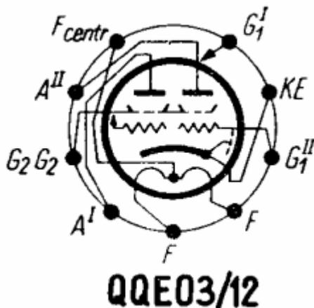
As the socket diagram shows, the screen grids of both sections are connected to pin 7.
