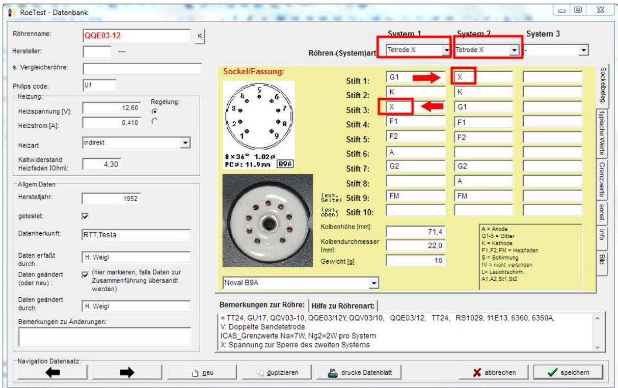
The tube type "Tetrode X" is selected for both systems. As you can see, as each section is measured, the control grid of the other section is connected to the X negative-voltage source.
