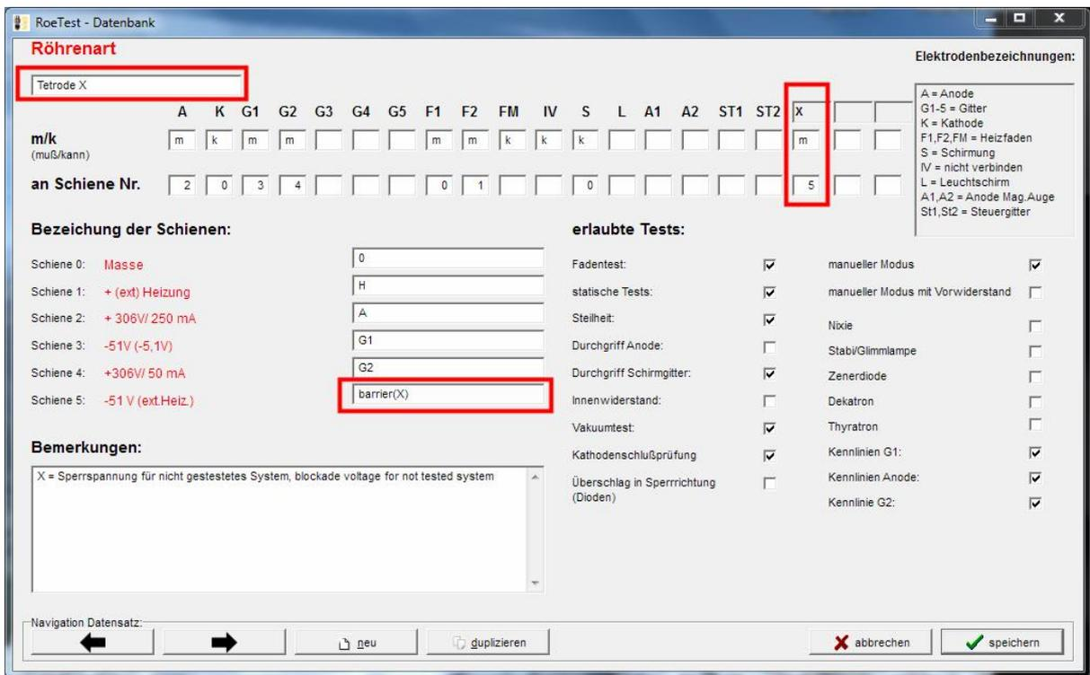
Here an electrode (X) is defined. This electrode is assigned to rail 5 (the second negative-voltage source in RoeTest).
