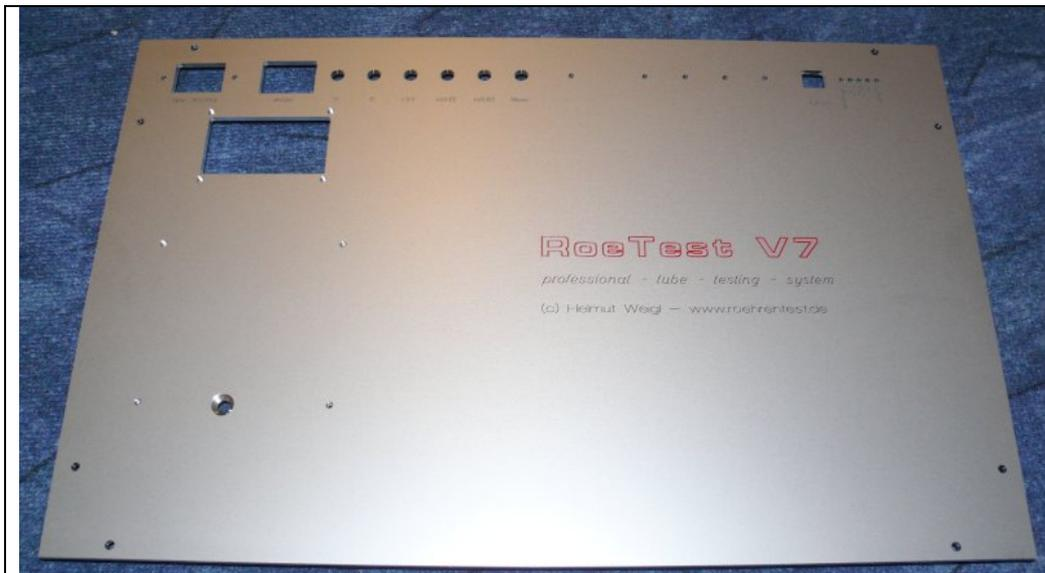
Front panel made by Fa. Schaeffer AG (made from 3 mm thick or more aluminum panel)
