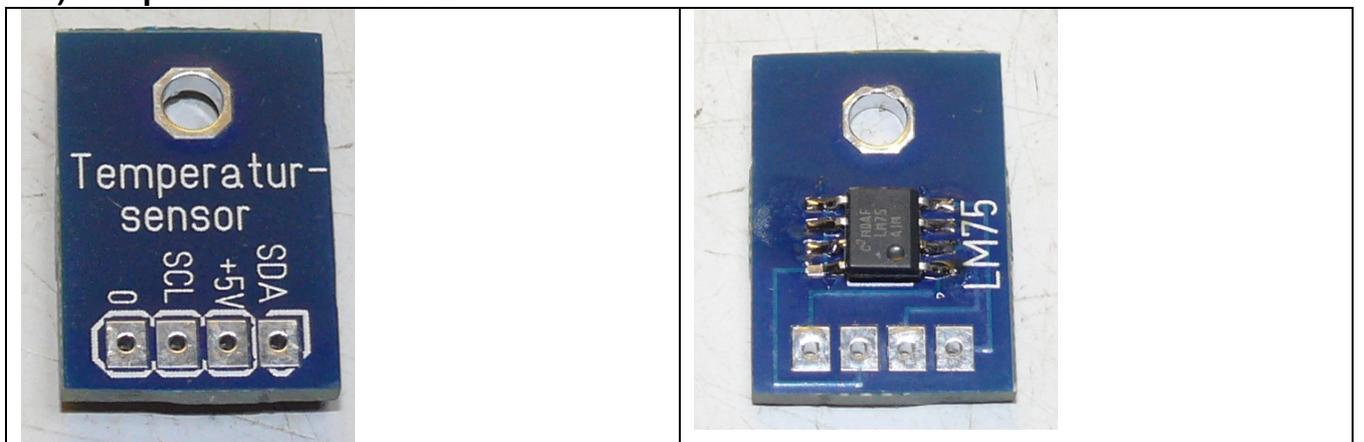
This PCB must be mounted to the heat sink in such a way that the LM75 IC touches it. I recommend the use of thermal compound between the IC and the heat sink. Be sure to insulate the pins to heat sink.
