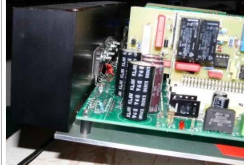
The front panel has a thickness of 3mm.
