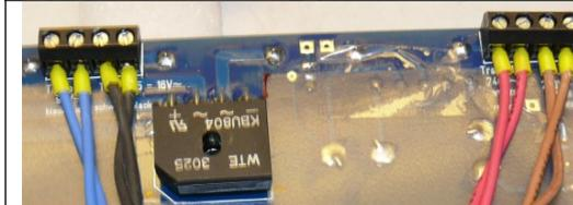
Solder the transformer wire connectors to the bottom side of the main board, for those wires routed in between the board and the front panel.
