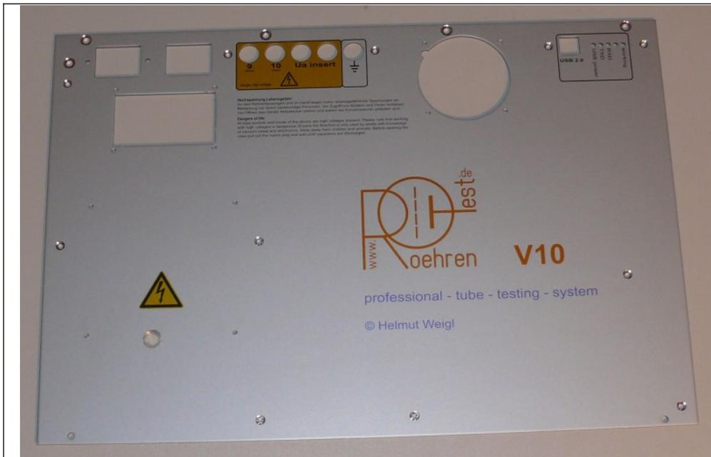
Front panel (V10) professional quality, manufactured according to my specifications by a leading German manufacturer, 3 mm aluminum, under anodized print (smudge-proof and scratch-proof, oil- and thinner-resistant), also anodized edges, cutouts and drill holes perfectly fitting
