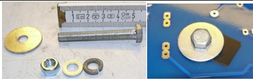
Please fasten the transformer's screw carefully. The colors of the secondary wires are printed on the PCB. For the primary connections see below.
