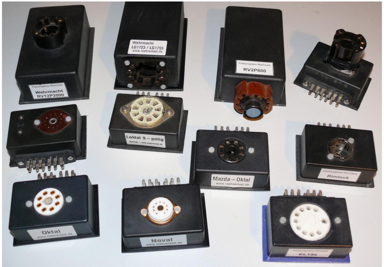
*Here are some examples of the tube socket boxes I'm using. The low cost plastic boxes get new bottom plates that are wider than the box itself (in my case it's 80 mm wide) so they fit into the rails of the socket box receiver.*
