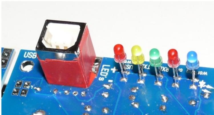
**Isolate the metallic case of the USB jack from front panel with a tape (black).**
