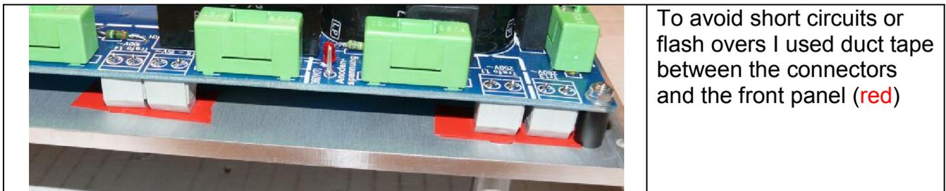
To avoid short circuits or flash overs I used duct tape between the connectors and the front panel (red)
