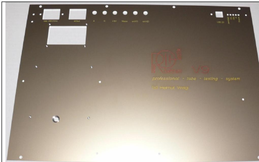
Front panel made by company Schaeffer AG (made from 3 mm thick or more aluminum panel)
