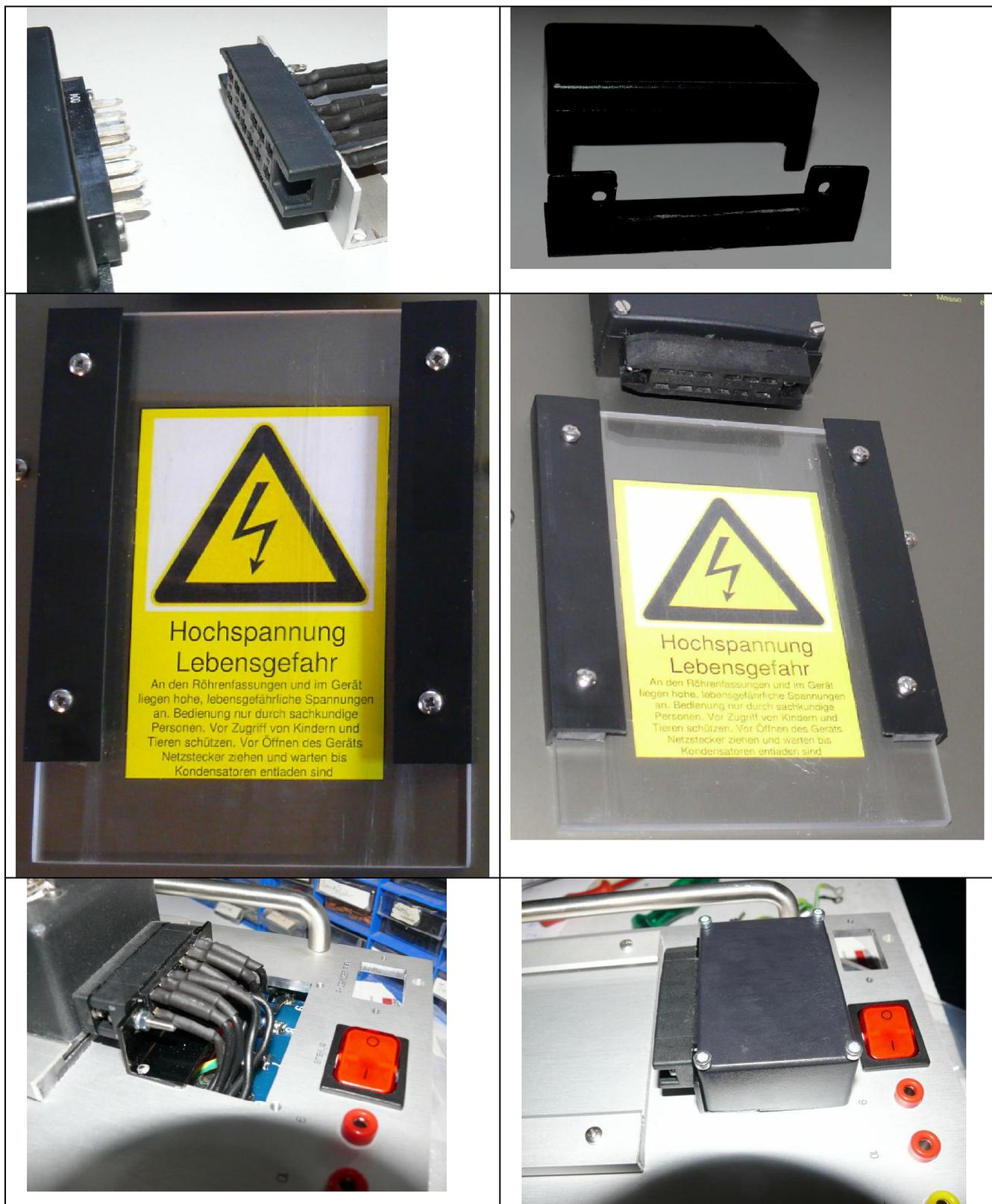
*The socket box receiver is made from plastic (clear acrylic or similar) and an aluminum or plastic angle and has two rails to guide the socket boxes. Make sure that the bolts are not too long and don't touch the PCB or the main transformer. Make sure to bolt the main transformer to the front panel before bolting on the socket box receiver.*
