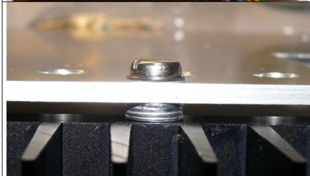
Attachment of heat sink to front panel with 4 screws M4x16.
