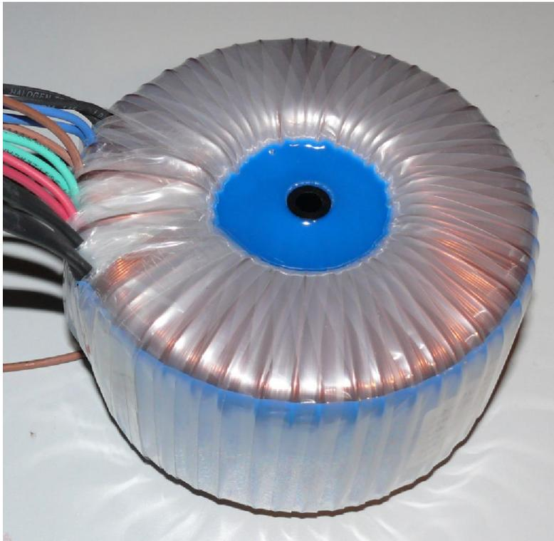
*Main transformer = toroid transformer (made to specification)*
