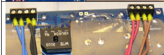
Solder the transformer wire connectors to the bottom side of the main board, for those wires routed in between the board and the front panel.
