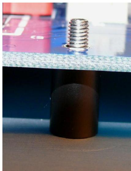
Attachment of mainboard to the front panel:
