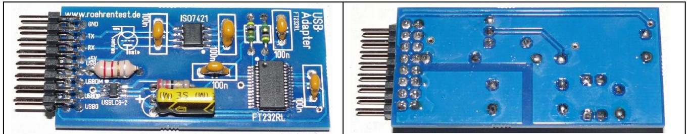
The USB interface is located on a **separate board that is plugged onto the mainboard**. USB female jack and the LEDs are located at the upper left edge of the mainboard.
