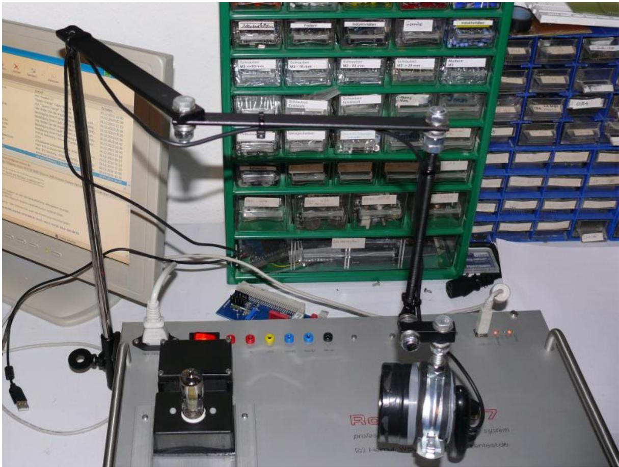
My monopod is simply made of some flat iron and round iron tubes, threaded rods and a bunch of nuts, bolts and washers. The monopod is attached using a pipe clamp.
