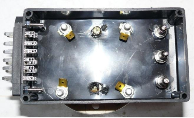
Then I fastened the socket contacts with through-going screws and soldering lugs. This way you can connect the contacts from the bottom and do not need wires running on the outside of the socket box.
