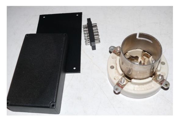
At first I dismounted the large socket and cut off the connection lugs so that they do not protrude on the sides any longer.
