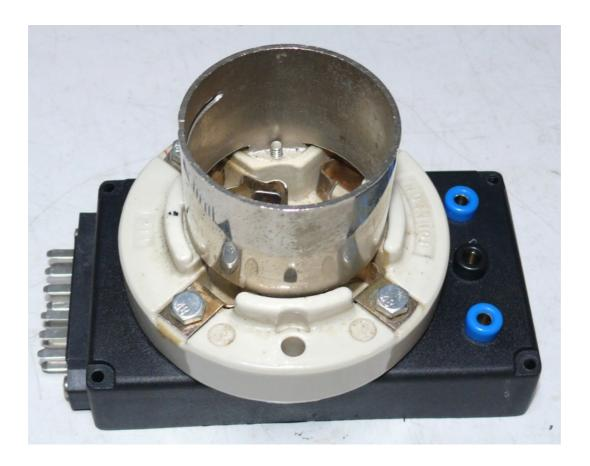
Note: The contacts should also be insulated. At the banana jacks an external heater supply can be connected.
