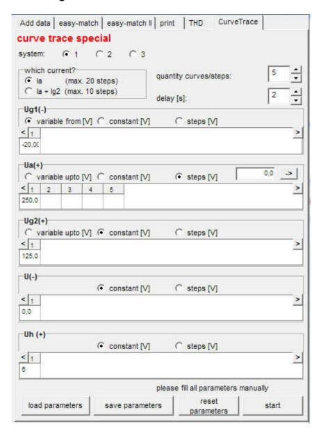
System: Specifies for which of the up to 3 tube systems characteristic curve recording shall be performed.
