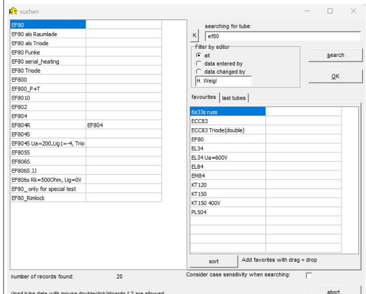
In the 'searching for tube' field, type the initial letters of the tube name (e.g., ef80) and press the return key (or the <search> button). All tubes that meet the search criteria are listed in the left-hand table.
