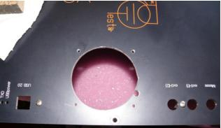
Mount the fan and the protection grill on the top side of the front panel. The fan's flow direction shall be from the housing's interior outwards through the front panel. This is also the air flow direction for natural convection. Caution: Assure that the fan's mounting screws do not stand out of the front panel's inner side and do not touch the main board.
