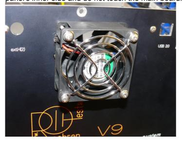
Connect the fan to the following socket on the main board (temperature controlled, switched by software):
