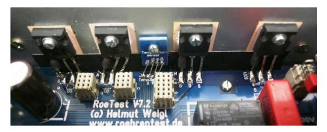
An aluminum cooler with about 1K/W it mounted onto the outer side of the back panel to dissipate the heat of the regulator transistors:
