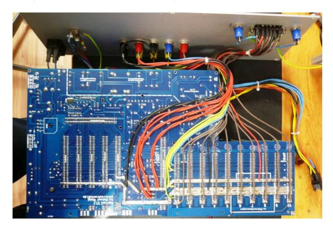
It took me about 35 hours to produce and integrate the cabling of the system. At this point the additional efforts for a system differing from the original design are heavily increased as well as for all the mechanical adaptions. The original design with the front panel as system carrier can be rebuilt much faster and more efficiently, also as it does not need these cable trees.
