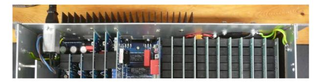
Beside the cooler there is a small fan transporting heat out of the housing, as soon as the thermal sensor has reached the adjusted temperature limit.
