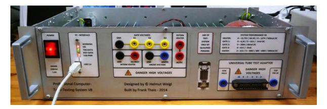
Here you can also see the experimental plugs for tube experiments using the system as a high end luxury power supply. This works extremely good with this system as you can control and watch all the voltages and currents in manual mode. And everything is perfectly protected then. I love it!
