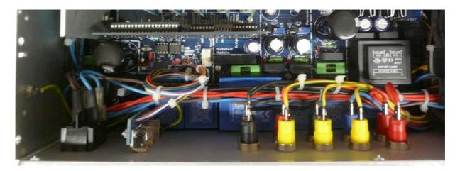
On the bottom side of the main pcb the wires for all tube signals are directly soldered to the board, fixed by hot-melt adhesive and then led to the front panel like this:
