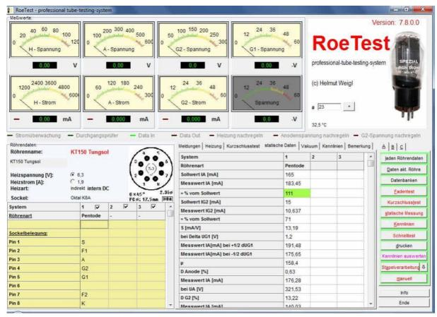
In many repeated single test cycles I tried to evaluate the reproducibility of the test results. Repeating tests with the very same tube for many times are only influenced by one parameter: the preheat time. Using different preheat times can change the test result by 5-10% (old tube designers experience).
