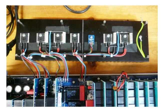
From the left to the right we now have: G2, Heater1, Heater2, 600V, T-Sensor, Anode1, Anode2
